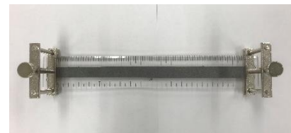
Figure 1. The resistor consists of CNP, two stainless steel pinchcocks, and a plastic ruler.
