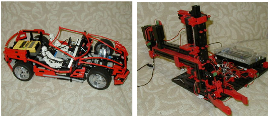
Figure 1. (Left) A Lego mobile robot in the form of a prototype car modified to hold an RCX with three motors and four sensors to control steering. (Right) A Fischertechnik industrial robot arm with articulated joints.
